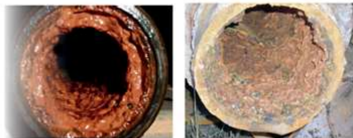
Figure 4.1: Scaling due to limestone deposits.
