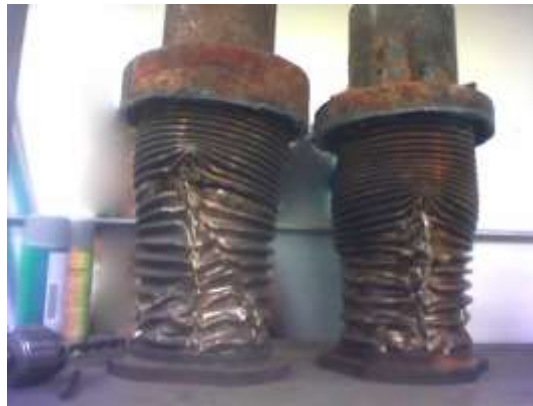
Figure 5.14: Expansion joint destroyed by water hammer
